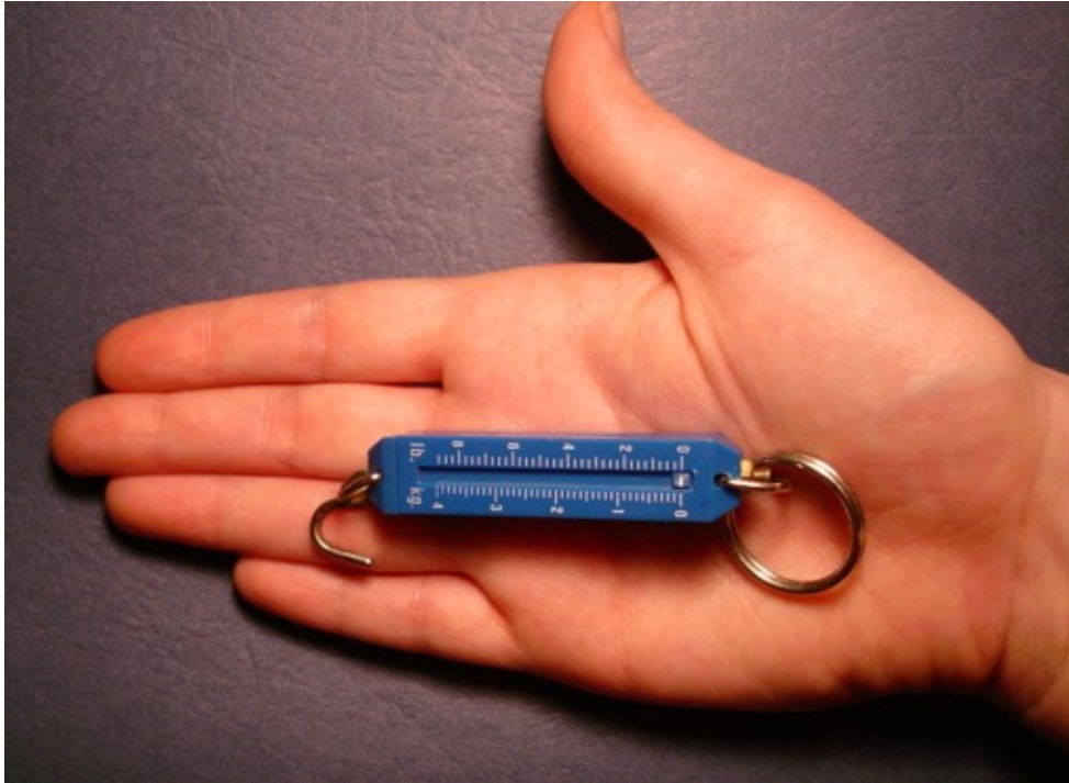
Figure 6. Hand scale used to weigh waste samples
