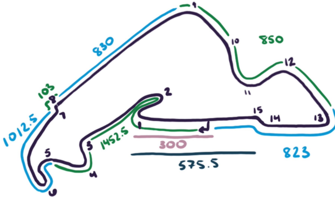
Figure 14: Rough circuit design following averages and turns of circuits from Table 3
